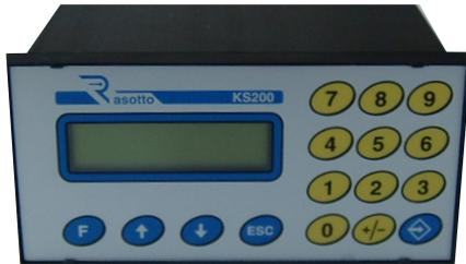
The KS201 is a single-quota positioner. The selection of the quota to be reached takes place via the keyboard setting (KEY F). When the start is pressed, the instrument automatically performs the quota by acting on the 4 relay outputs. By moving the axis in manual mode the instrument works as a meter and displays the value supplied by the encoder.
